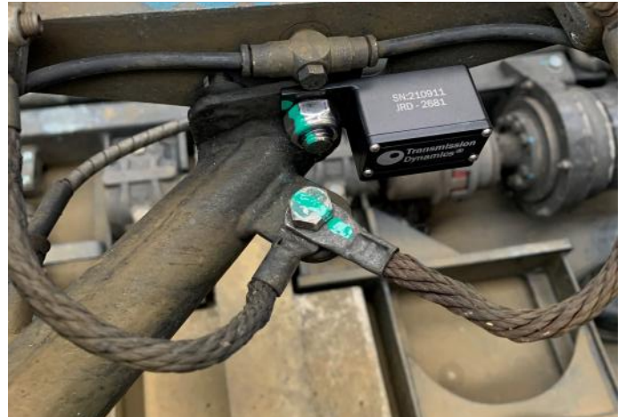
PANDAS® Wireless Accelerometer bracket assembly
