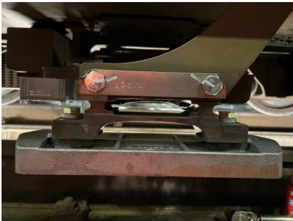
Figure 1. Wireless Accelerometer mounted on shoe gear
