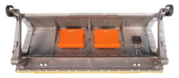
Transmission Dynamics has developed the SmartStep® system, an advanced in-service data logger that monitors escalator performance, automatically reporting potentially damaging events in real time. The system consists of a battery-powered data logger with wireless communication, integrated into a standard escalator step. It operates autonomously for up to a year (between battery changes), alerting operators to abnormal conditions.
