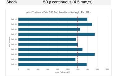
The above graph shows the axial preload of 10off bolts monitored by the LoRa LMF+. The red vertical line is the minimum permissible preload threshold, so 2-off bolts have generated a report sent via email to key stakeholders.
