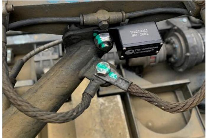
PANDAS® Wireless Accelerometer bracket assembly
