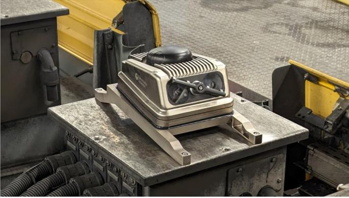
PANDAS-V® camera installed on a train roof
