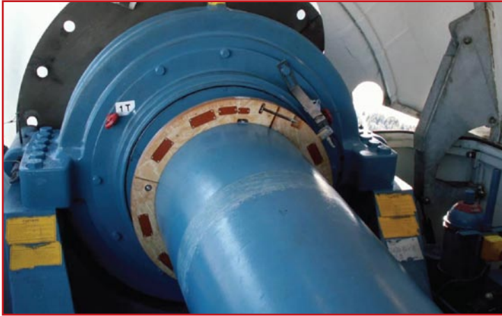
Fig. 4: Input shaft equipped with Transmission Dynamics' torque monitoring equipment.
