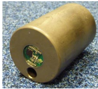
Fig. 17: Rolling element with embedded face load intensity distribution measurement system. High-speed telemetry system operates at 80 ksps, 12-bit SHH and is powered from an integrated miniature battery.
